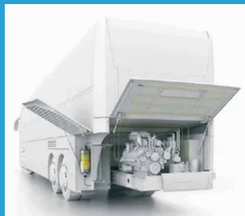
Bus Fire Suppression System
